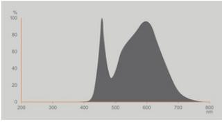
EPREL Data Spectral Diagram LEDr
